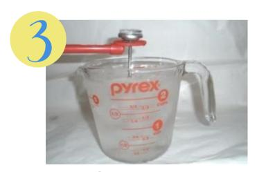
Insert thermometer stem & make sure the dimple is submerged.
